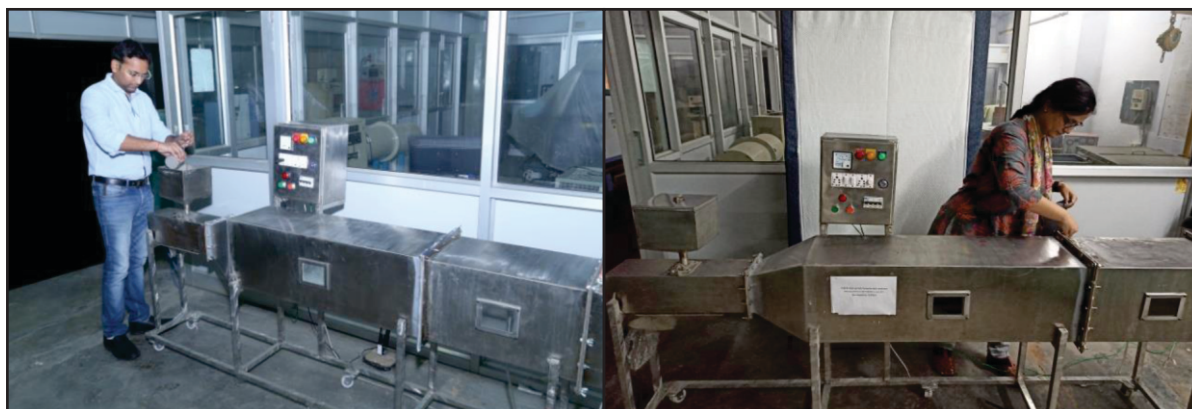
Fig.2: NITRA - Fabric dust resistance tester (Indian Patent application no. 201711002704)
