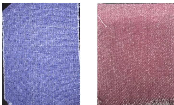
Fig. 7 : Cotton Fabrics having denim effect created by using disperse dye
