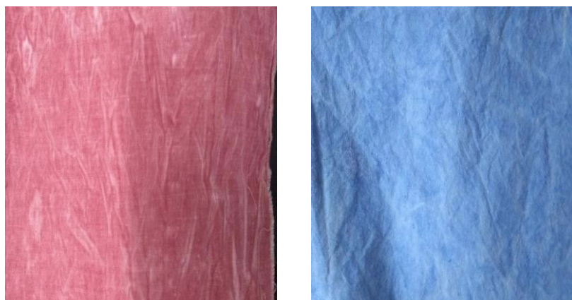
Fig. 6 : Cotton Fabrics dyed in solid shades using disperse dye
