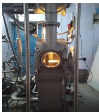
Fig. 4: Soft flow dyeing machine used for cotton hank dyeing.
